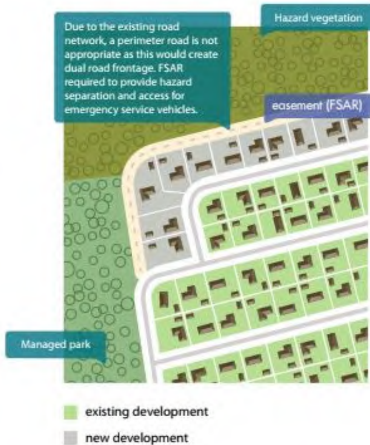
Figure 26: Example of a fire service access route
