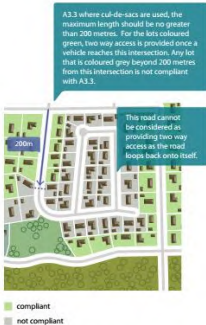
Figure 21: Example of compliant and non-compliant two-way
